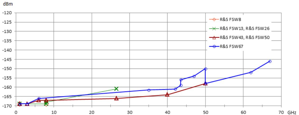
Typical displayed average noise level of the R&S®FSW models for  $f > 1$  GHz with R&S®FSW-B24<sup>7</sup> RF preamplifier option, preamplifier gain = 30 dB.
